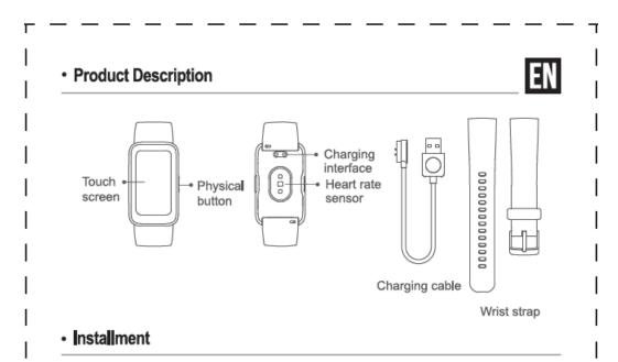
Insert the lugs on the wrist strap into the ear holes in the main body, until you feel and hear a "click", that is the installation is successful.
