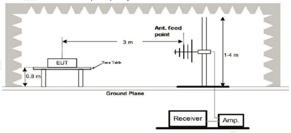
3. Radiated Emission Test-Up Frequency Above 1GHz
