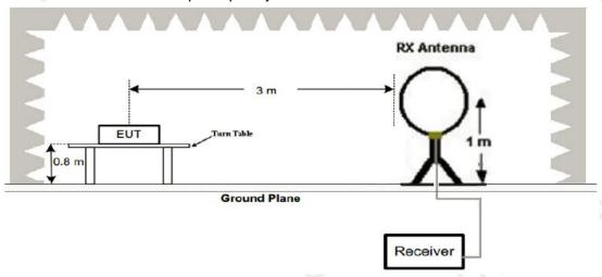
2. Radiated Emission Test-Up Frequency 30MHz~1GHz
