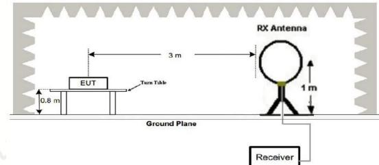
2. Radiated Emission Test-Up Frequency 30MHz~1GHz
