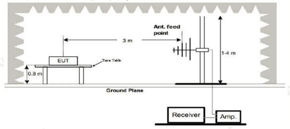
3. Radiated Emission Test-Up Frequency Above 1GHz
