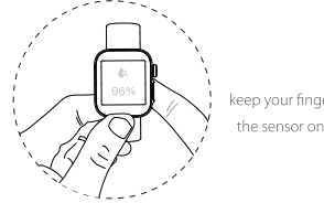
keep your finger pulp touch tightly the sensor on the bottom to test
