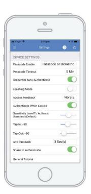
The two main configuration options for this are the "Sensitivity Level to Activate" slider, which determines how easily your mobile device with pick up the activation zone, and the "Anti Passback" setting, which defines the number of seconds between each attempt to resend a mobile credential. To adjust these settings, select the 'Settings' tab
