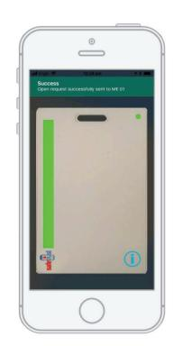
To open the door, simply present your mobile device running the Safetrust Wallet application to the SABRE Module. When the phone is within the configured activation range, the LED within the assigned credential for this identity system will be green in color. If "Auto Authenticate" is enabled for the mobile credential, the credential will be sent to the SABRE Module whenever the mobile device is within the activation zone.
