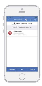
With the Admin Installer tab open from the App, bring the phone in range of the SABRE Module and once visible from the App, highlight and select "Configure".
