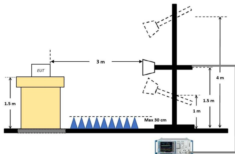
**TEST PROCEDURE OF RADIATED SPURIOUS EMISSION (BELOW 30 MHz)**
