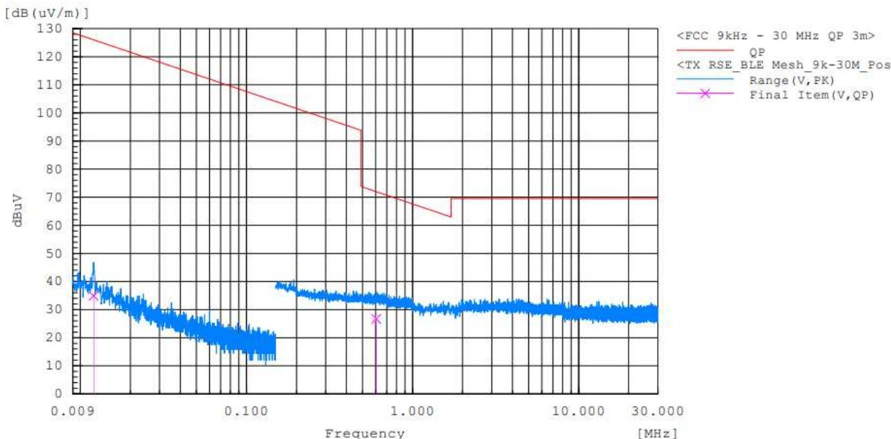
**Radiated Spurious Emission 9 kHz – 30 MHz (Antenna Position 180°) : BLE MESH (CH 39 : 2480 MHz)**
