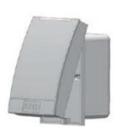
Once the screw is removed pull the reader out and up to remove it from the wall mount bracket.
