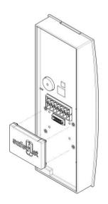
Position the SABRE module (with logo up), onto the Hirose connector and press firmly to make a connection.
