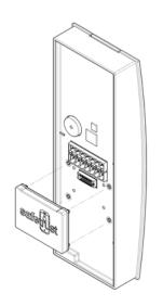
Position the SABRE module (with logo up), onto the Hiroshi connector and press firmly to make a connection.
