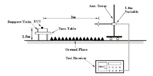
The radiated emission tests were performed in the 3 meters test site, using the setup accordance with the ANSI C63.10 - 2013. The specification used was the FCC 15  $\S$  15.209, 15.205 and 15.231.
