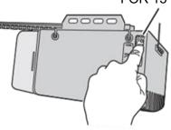
NOTE: PRESSING THE LEARN BUTTON FOR MORE THAN 10 SECONDS WILL ERASE ALL KEYPAD CODES AND REMOTE CONTROLS
