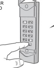
OPERATOR LIGHTS FLASH WHEN THE KEYPAD CODE IS ACCEPTED
