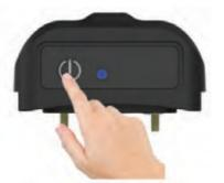
3. Press the power button 3 times on the receiver to enter the pairing mode. You will hear a beep and the LED indicator will become solid. You will now have 10 seconds to finish the pairing.
