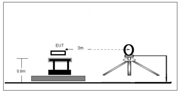
(B) Radiated Emission Test-Up Frequency 30MHz~1GHz
