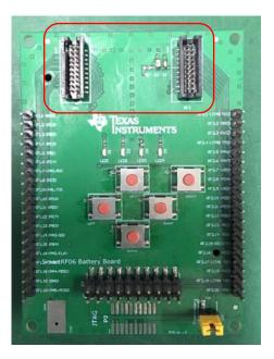
The module insert the mainboard according to the requirements of customers, pay attention to the position, the user inserts the needle should be vertical and gently, otherwise it may cause deformation of pin module.
