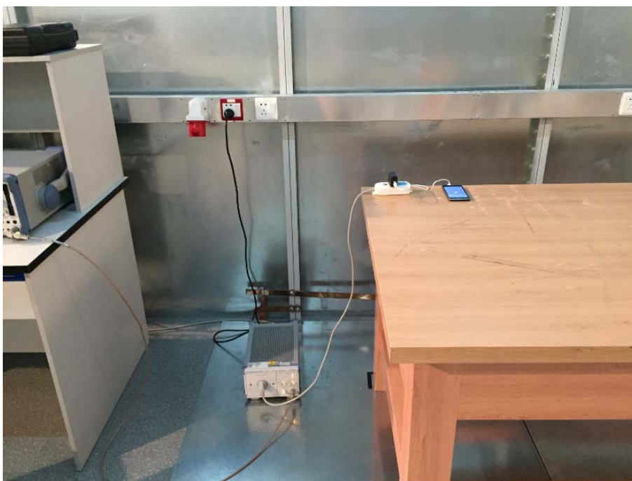
Conducted Power Line Emission test
