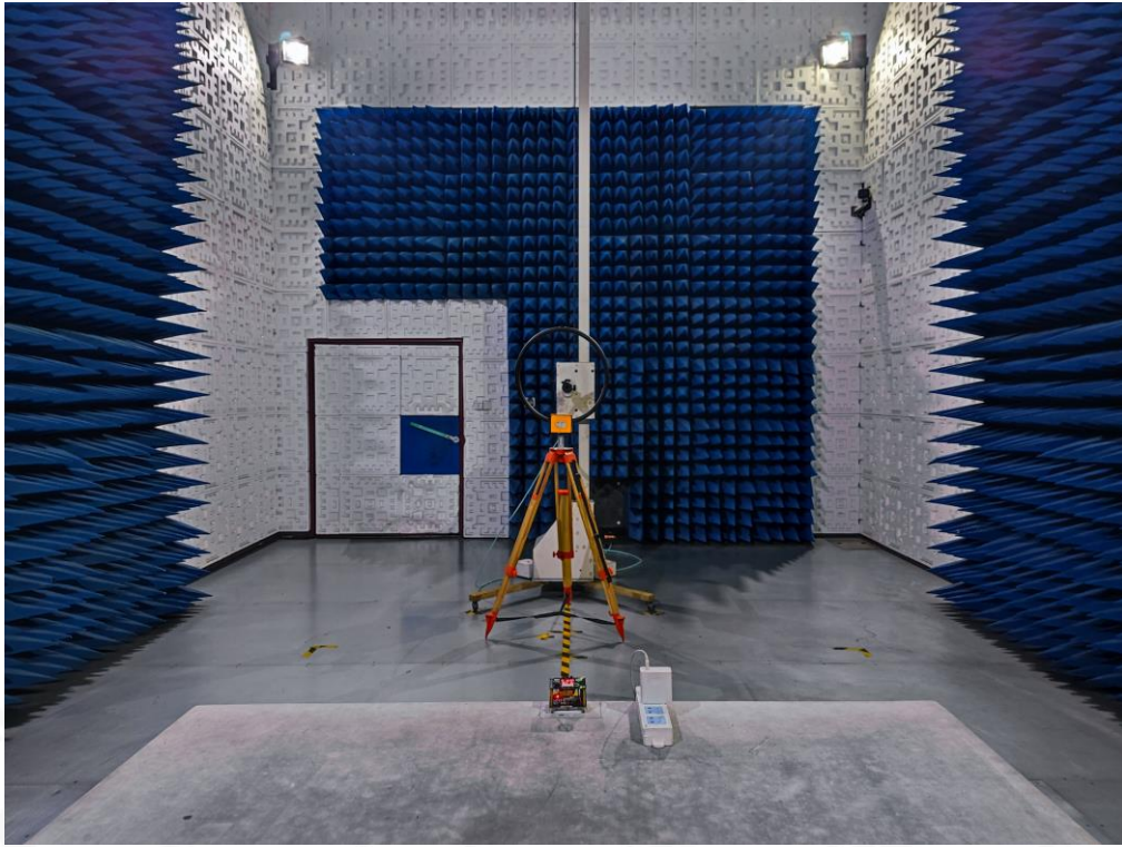
RADIATED EMISSION TEST SETUP 30MHz-1GHZ
