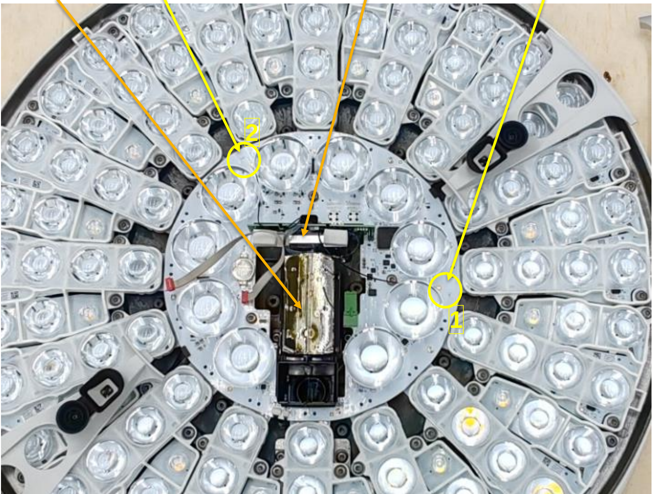
Camera System Position PCB antenna2 WL.V.TX with Heatsink at AMNPTTX01 Position PCB antenna1
