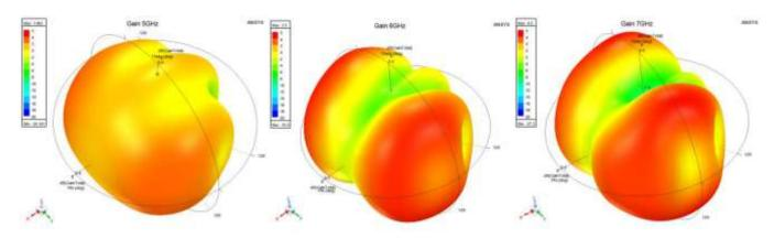
Note that with a different PCB length, the radiation can be directed more to boresight (+x direction).
