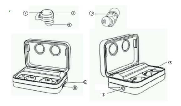
①touch control panel ②microphone ③earphones charging contacts ④ear cap ⑤power button ⑥type-c input port ⑦charging case contacts ⑧wired headphone jack
