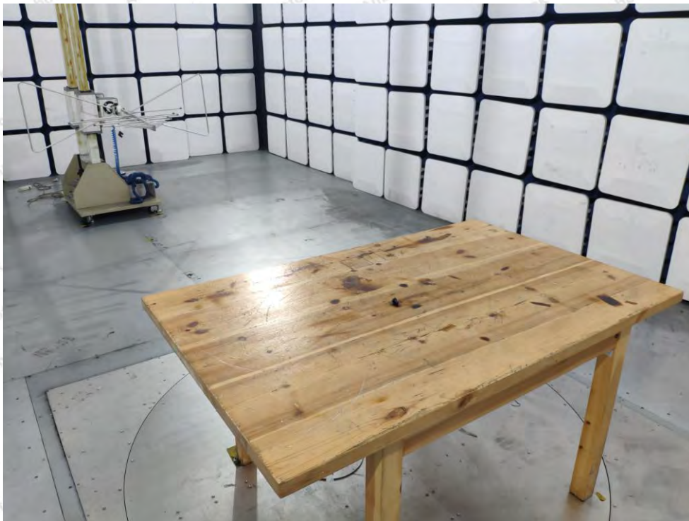
Photo of Radiation Emission Test
