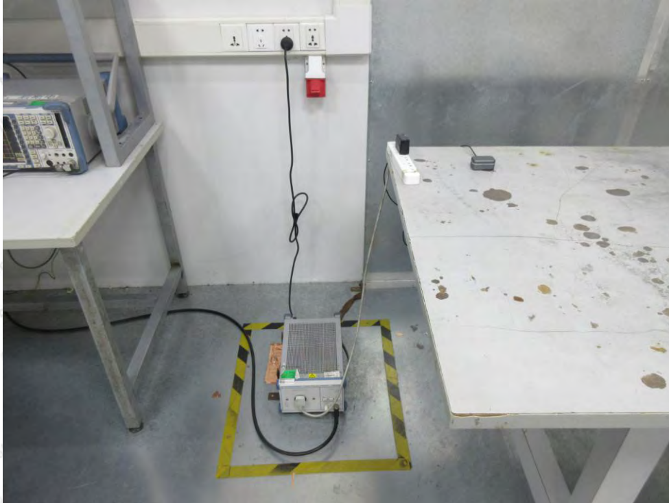
Photo of Power Line Conducted Emission Test
