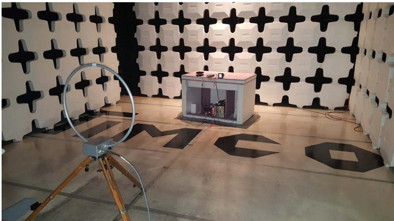
FIELD STRENGTH SPURIOUS EMISSIONS  $f < 200\text{MHz}$
