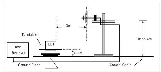
(c) For radiated emissions above 1000MHz
