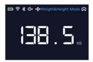
4.After the weight measurement, wait for the voice prompt to take the height measurement. Follow the voice and screen prompts, stand up straight, wait for the height measurement result number to remain stable on the screen, then the height measurement is completed, at this time, your height data will be displayed on the screen.
