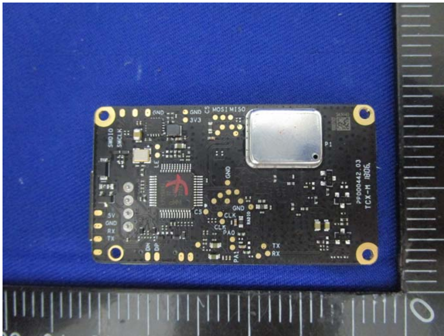
EUT –Wireless Module RF Board Bottom View
