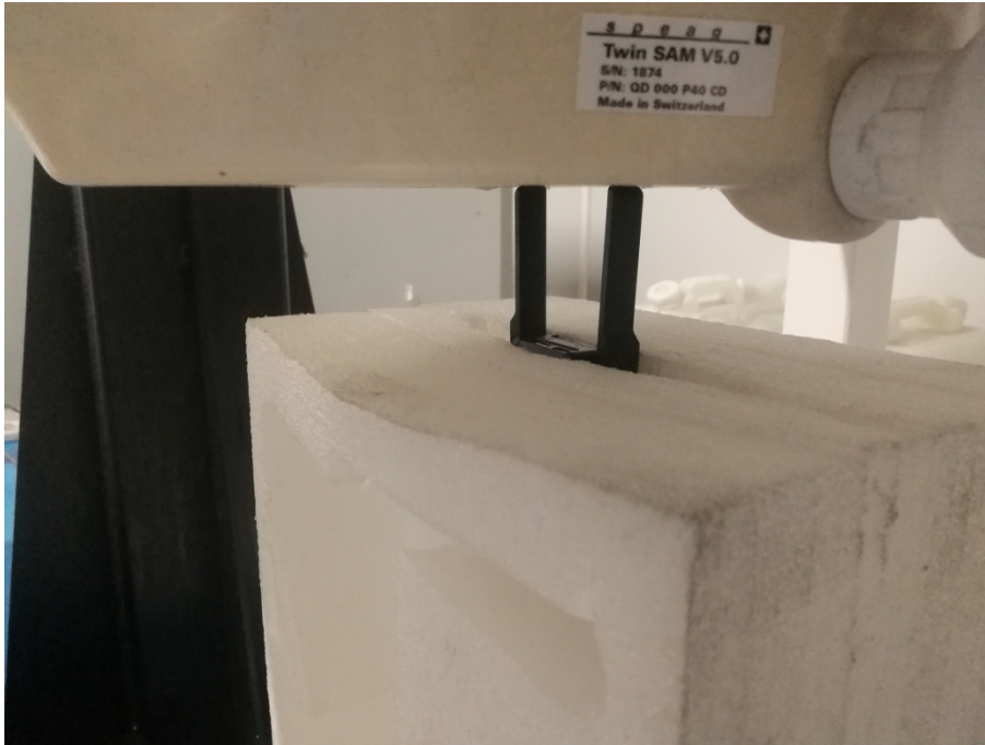
Extremity(Hand) With Antenna Unfold Setup Photo(0mm)
