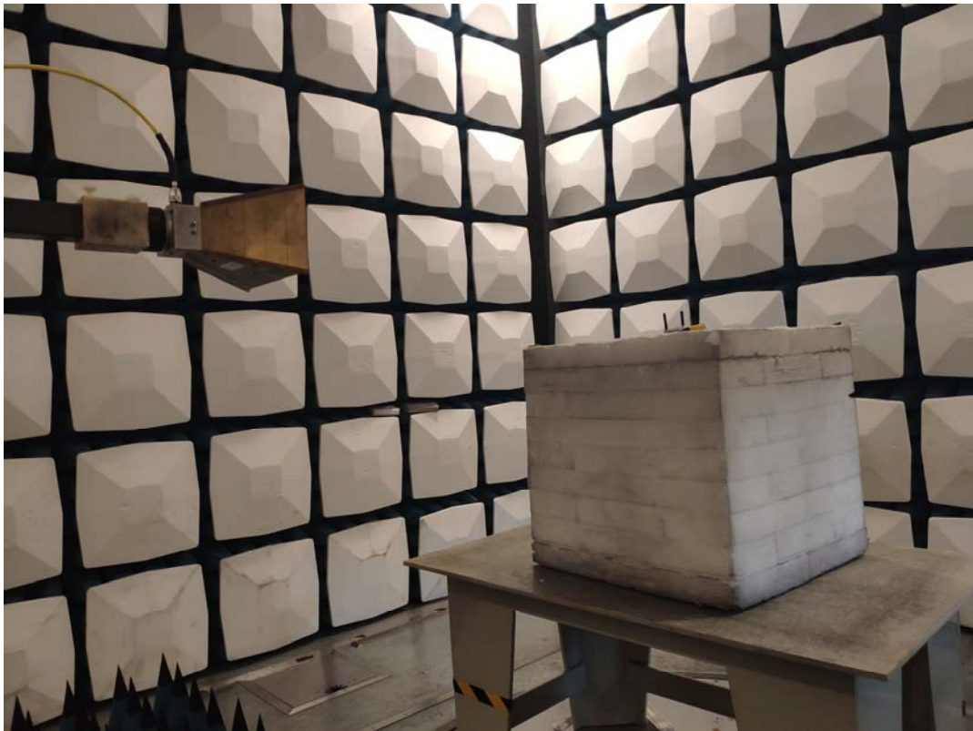
Radiated Emission Above 1GHz View
