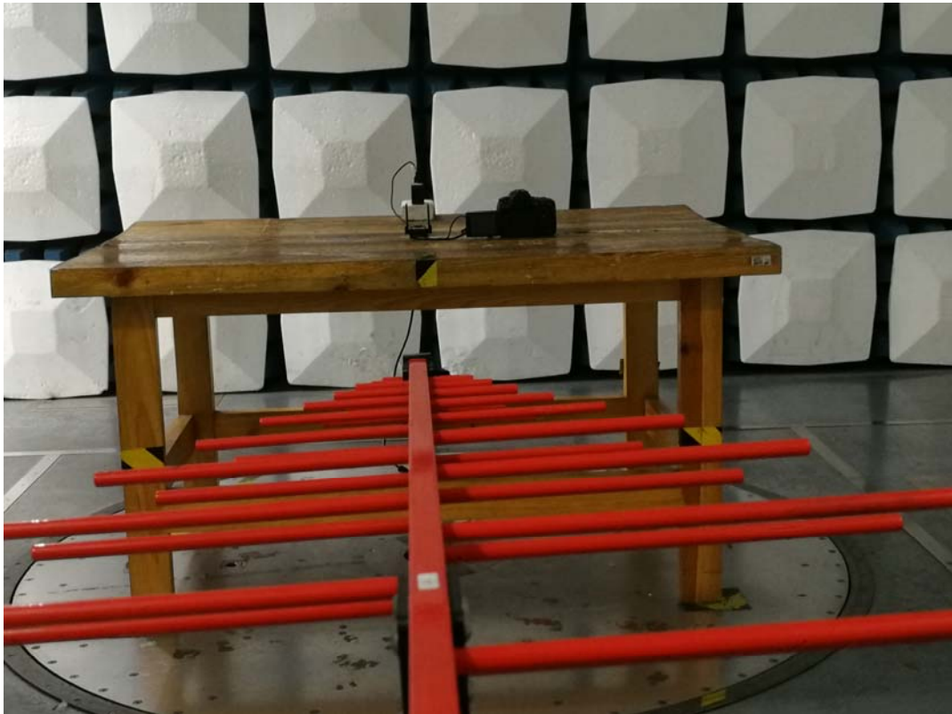
Radiated Emission Above 1GHz View
