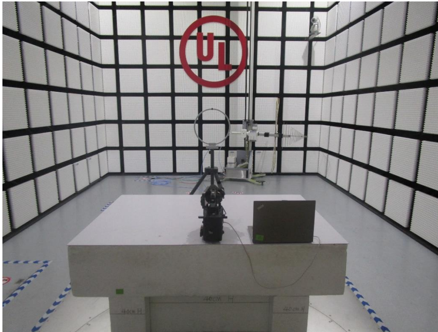
RADIATED RF MEASUREMENT SETUP (Below 30MHz)
