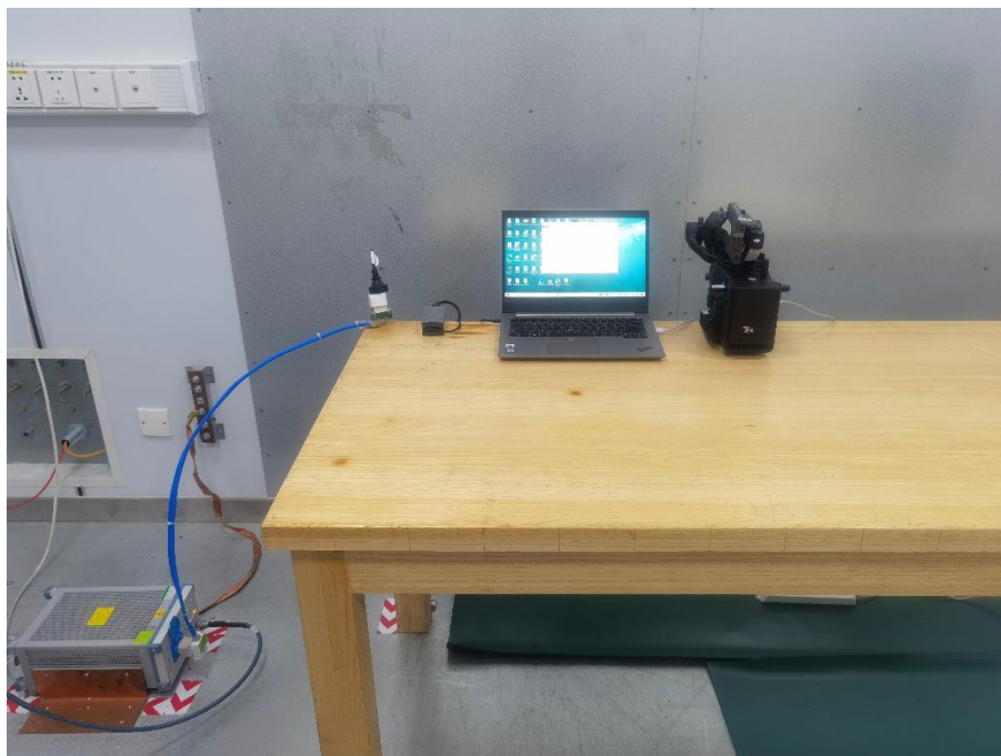
POWERLINE CONDUCTED EMISSIONS MEASUREMENT SETUP
