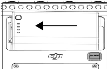
2. Press the power button on the left side of the monitor to power on once the battery is mounted. Refer to the DJI High-Bright Remote Monitor User Guide for more information on how to use the monitor such as activation, linking, and navigating the touchscreen interface.
