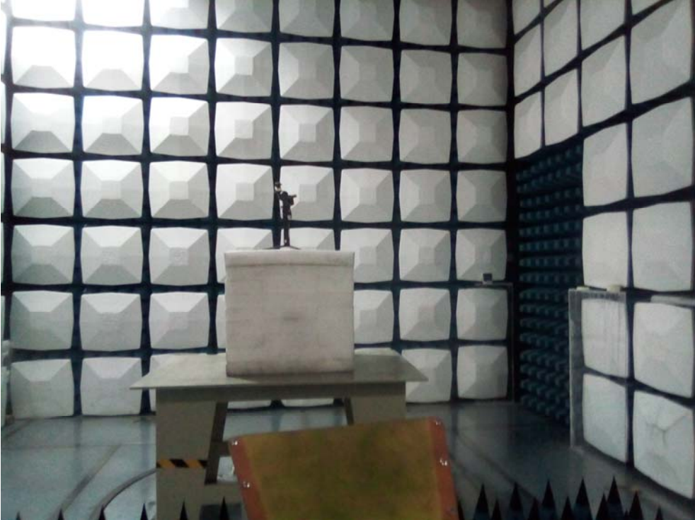
Radiated Emission Above 1GHz View
