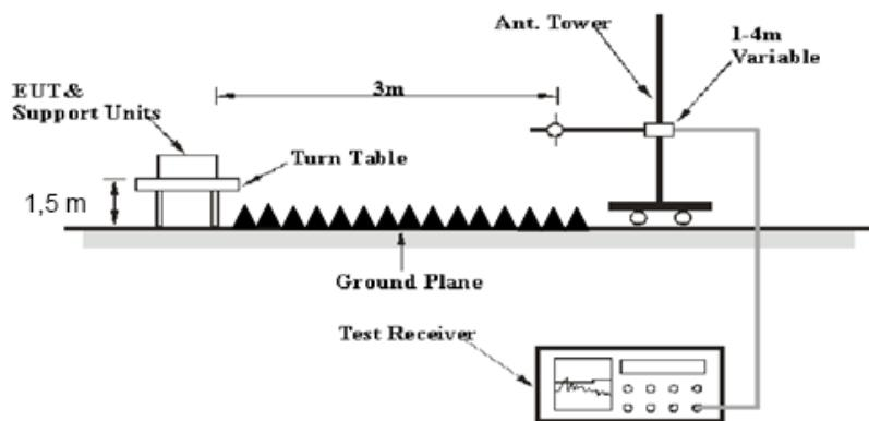
The radiated emission Below 1GHz tests were performed in the 3 meters chamber test site A, above 1GHz tests were performed in the 3 meters chamber B, using the setup accordance with the ANSI C63.10-2013. The specification used was the FCC 15.209, and FCC 15.247 and RSS-247 §5.5,RSS-Gen §8.10 limits.
