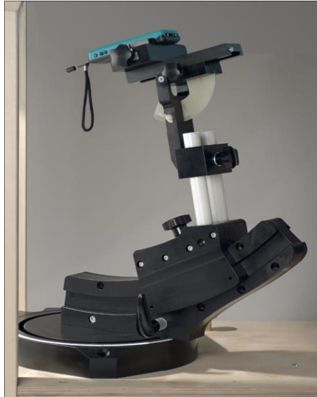
F-2. Device Holder for Transmitters
