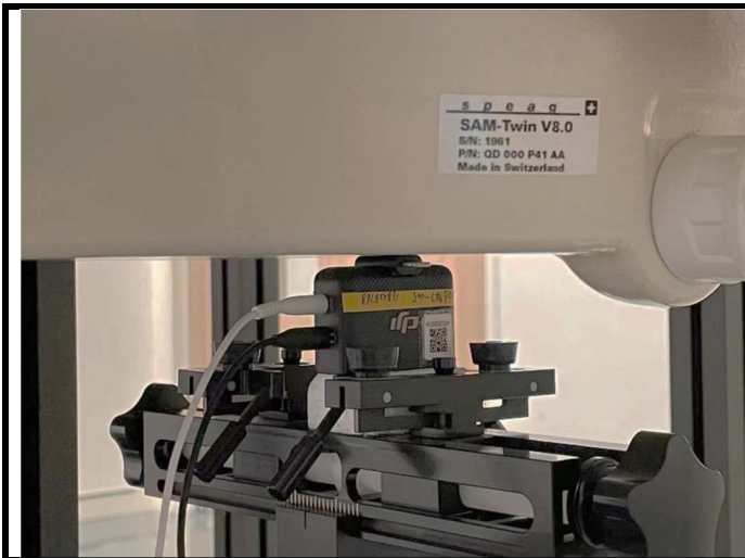
Rear Face of EUT + Earphone + Clamp with 0 cm Gap
