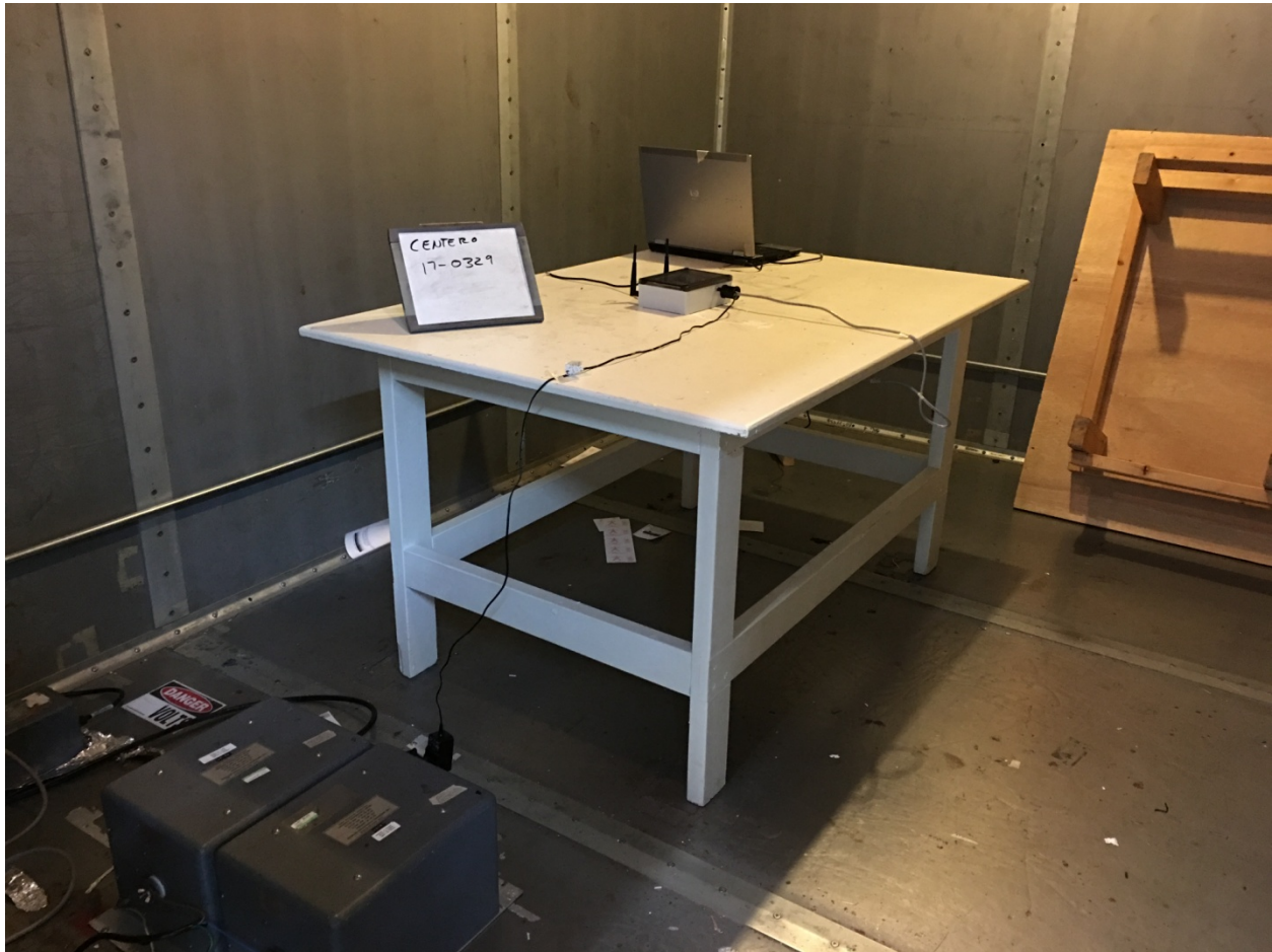
Figure 9. Powerline Conducted Emissions Test Configuration
