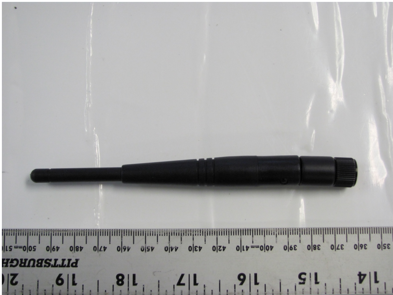
Figure 10. Antenna (both antennas are identical)
