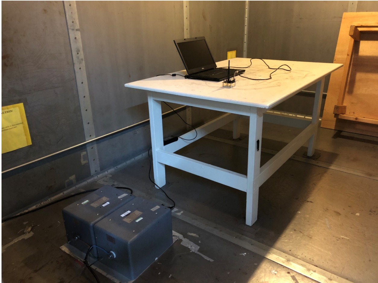
Figure 6. Power Line Conducted Emissions
