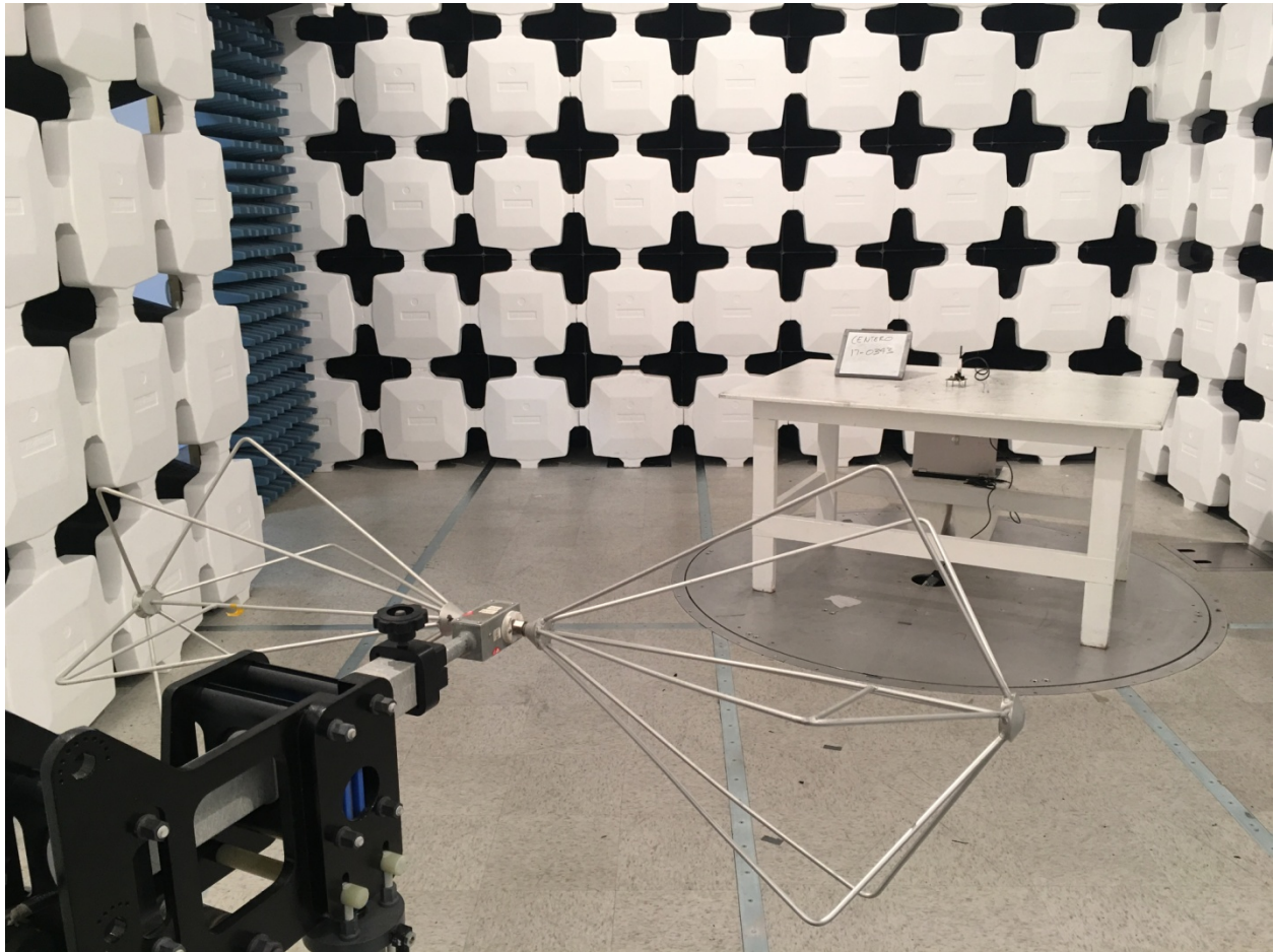
Figure 3. Radiated Emissions, 30-200 MHz
