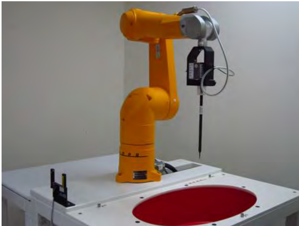
Fig.1 Photograph of the SAR measurement system
