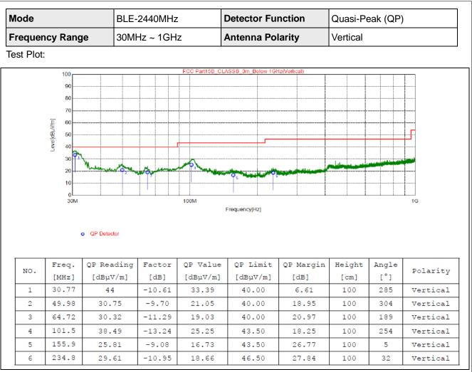
1. Emission Level(dBuV/m) = Original Spectrum reading (dBuV) + Correction Factor(dB/m)
