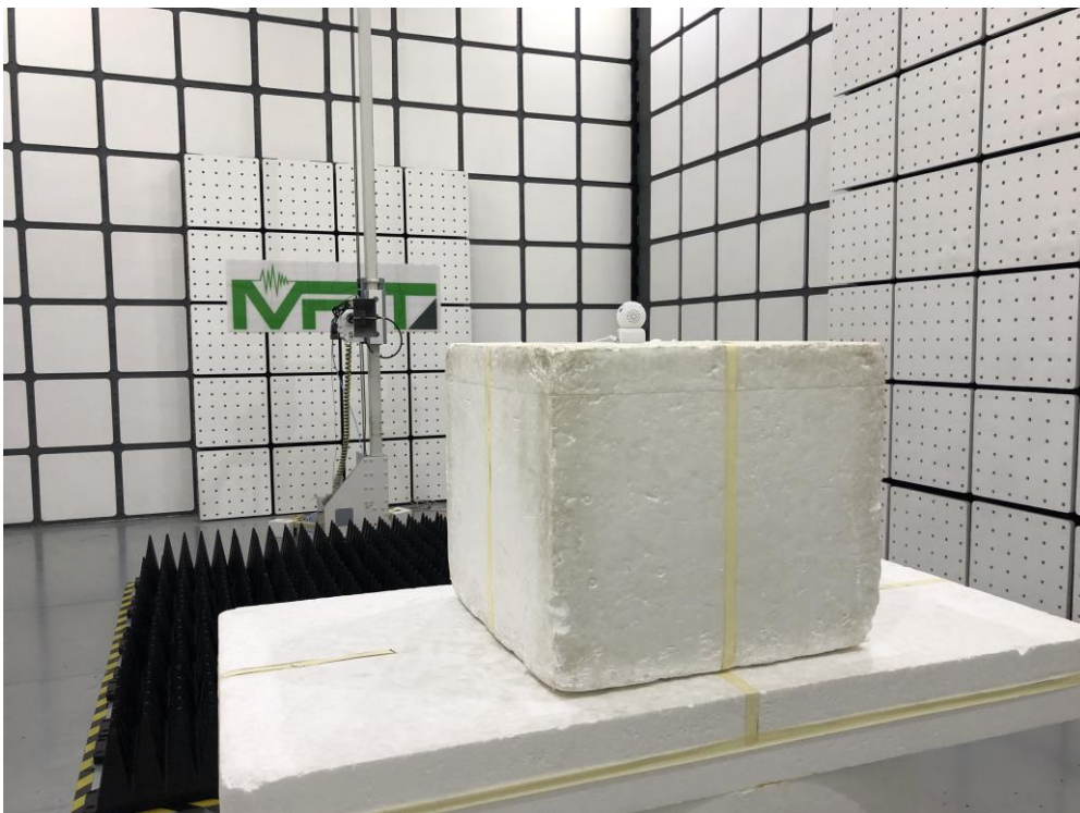
Description: Radiated Restricted Band Edge Test Setup (for 5G Wi-Fi)
