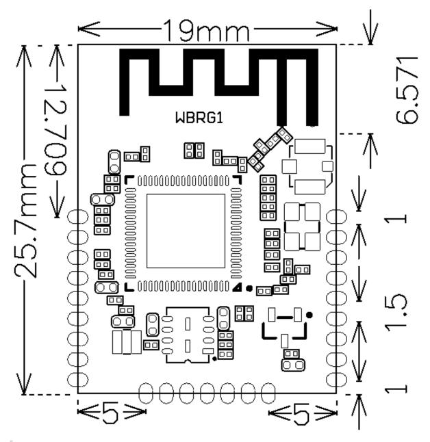
**Note**: For the PCB frame, the dimensional tolerance is  $\pm 0.35$  mm, and for the thickness of the PCB, the dimensional tolerance is  $\pm 0.1$  mm.
