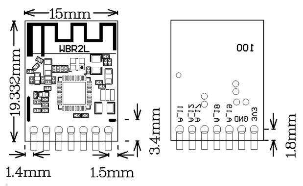
**Note**: The default dimensional tolerance is  $\pm 0.35$  mm. If you have specific requirements on dimensions, make them clear in the datasheet after communication.
