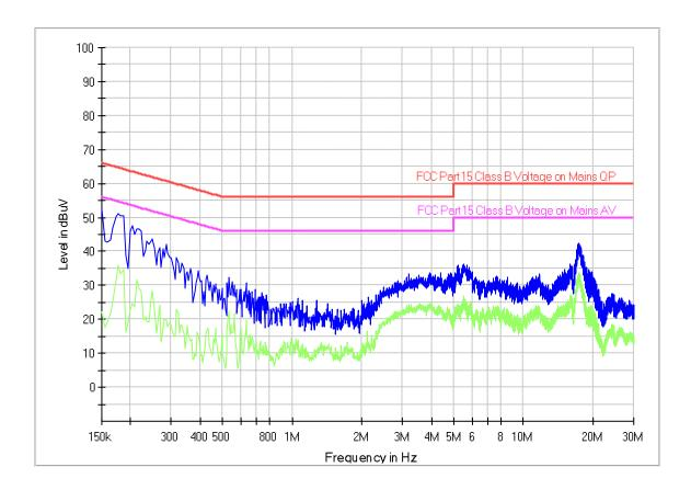
Note 1: Measure Level (dBuV/m) = Reading Level (dBuV) + Factor (dB) Factor (dB) = Cable Loss (dB) + LISN Factor (dB) + 10dB Attenuator
