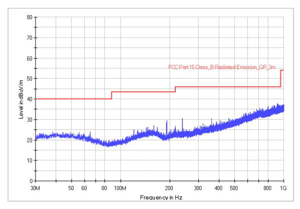
Note 1: Measure Level (dBuV/m) = Reading Level (dBuV) + Factor (dB)
