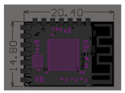
Figure 1. TYZS5dimensional drawing
