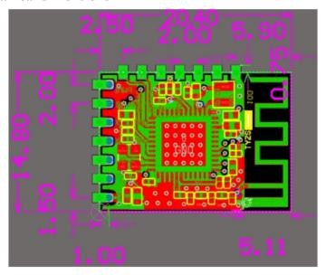
Figure 3: The TYZS5mechanical dimensional drawing
