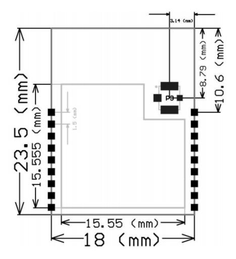
Figure 6-1 TYWRD1S mechanical dimensions
