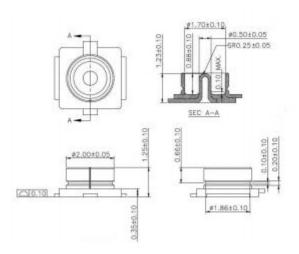
Figure 5-1 U.FL RF connector parameters
