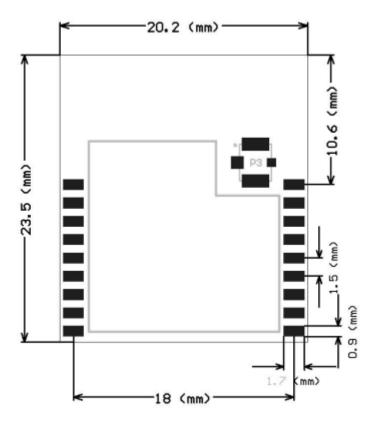
Figure 6-4 Layout of the PCB to which TYWRD1S applies
