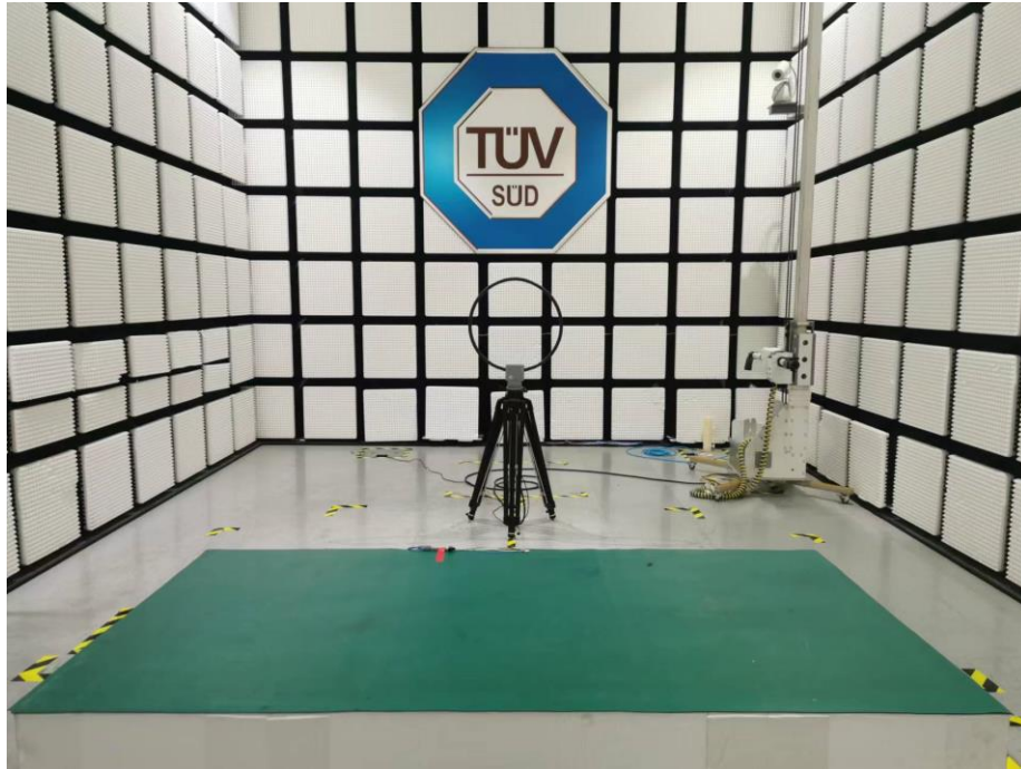
Radiated Emission Setup 9kHz ~ 30MHz
