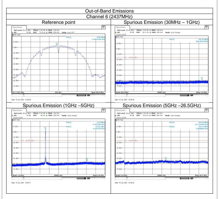
Note: The emission which exceed the limit is the fundamental.
