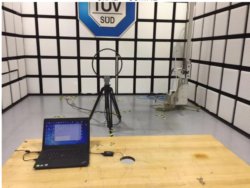
Radiated Emission Setup 9kHz ~ 30MHz
