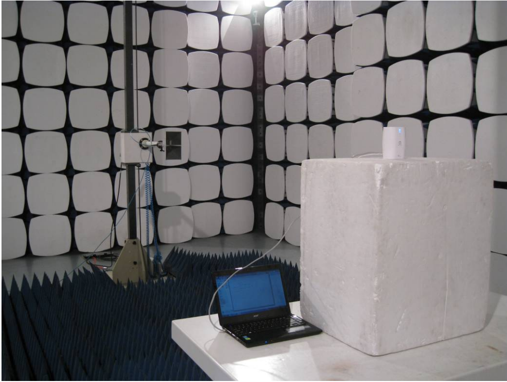
Radiated Setup photo (Above 1G)
