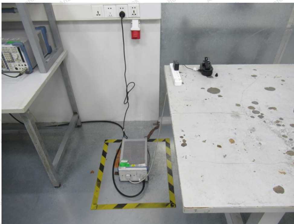
Photo of Conducted Emission Measurement
