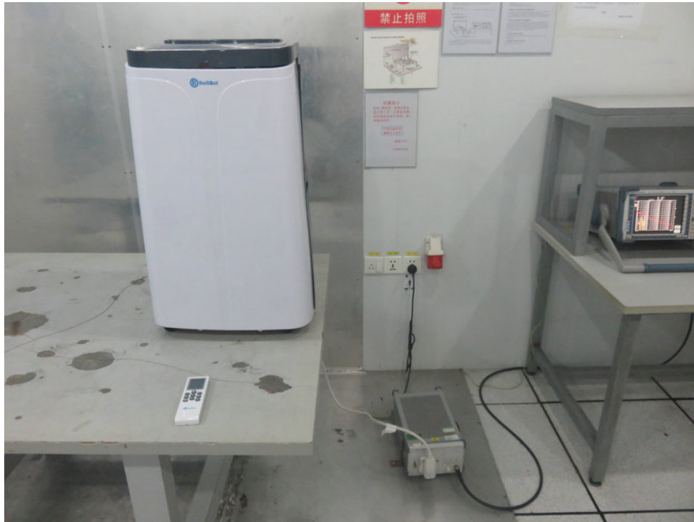
Photo of Conducted Emission Measurement
