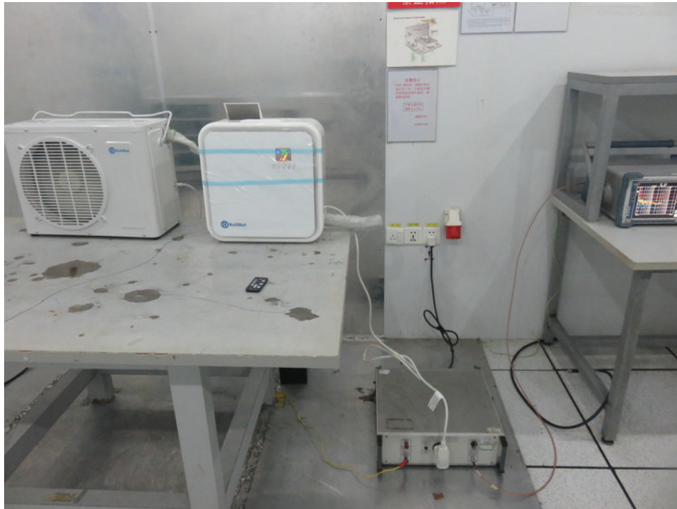
Photo of Conducted Emission Measurement
