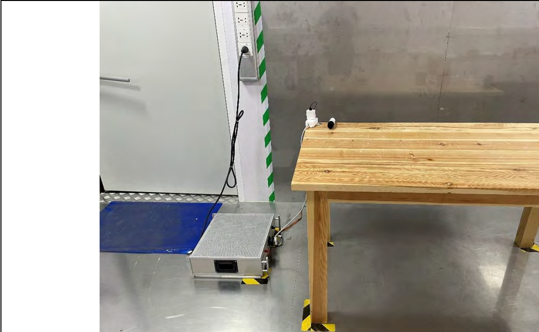
Conducted Emission at AC power line
